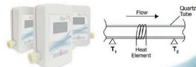
Figure 2: Scheme of Testa thermal flowmeter.
